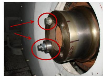
**Figure 8: Picture of the used balancing plane**
