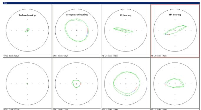
**Figure 18: Orbit plots at different load conditions (up 110MW ; down 330MW)**
