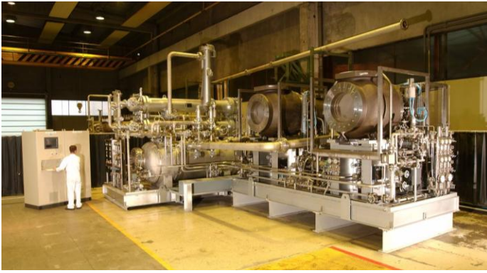
Figure 1. Dual turboexpander 2-TC 400/90 with the oil unit and control panel assembled in the workshop
